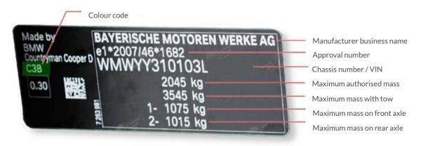
The manufacturer label is shown to be attached to the base of the right (driver-side) centre pillar. There are additional VINs located on the left side of the vehicle under the windscreen and die-cut in the turret on the suspension. The tyre pressure label is attached to the left (passenger-side) centre pillar.
